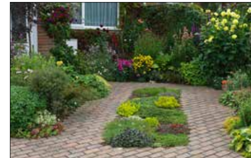
Example of limited paving to provide access and parking, combined with planting to create visual interest, biodiversity and permeability
